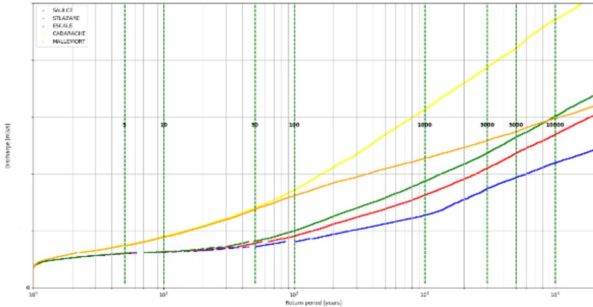
Figure 10. Discharge CDFs computed with AutoMaT and Durance River Mascaret model (with a test set of hydrographs) – blue: Saulce Dam, red: St Lazare Dam, green: Escale Dam, yellow: Cadrache Dam, orange: Mallemort Dam
