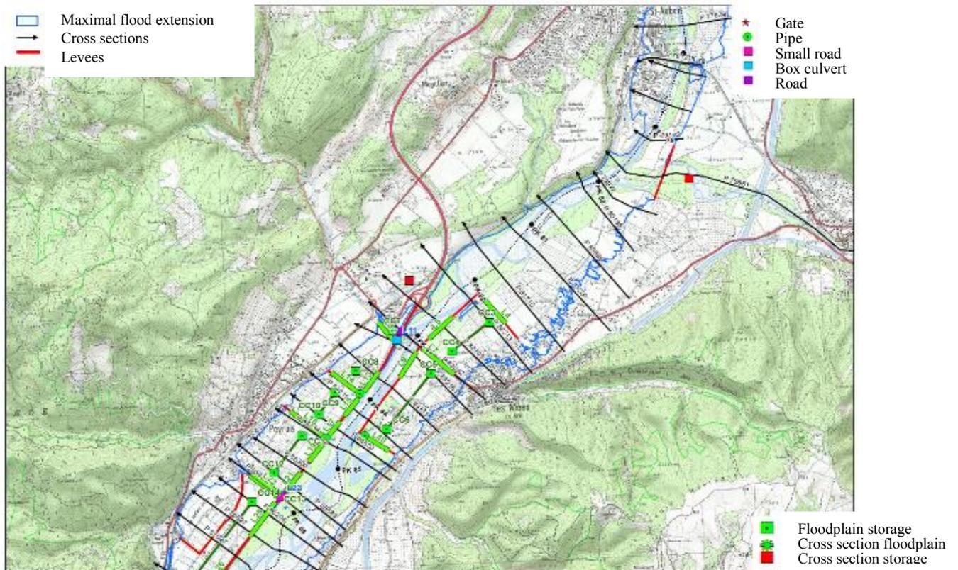
Figure 8. Scheme used to model Durance River with Mascaret
