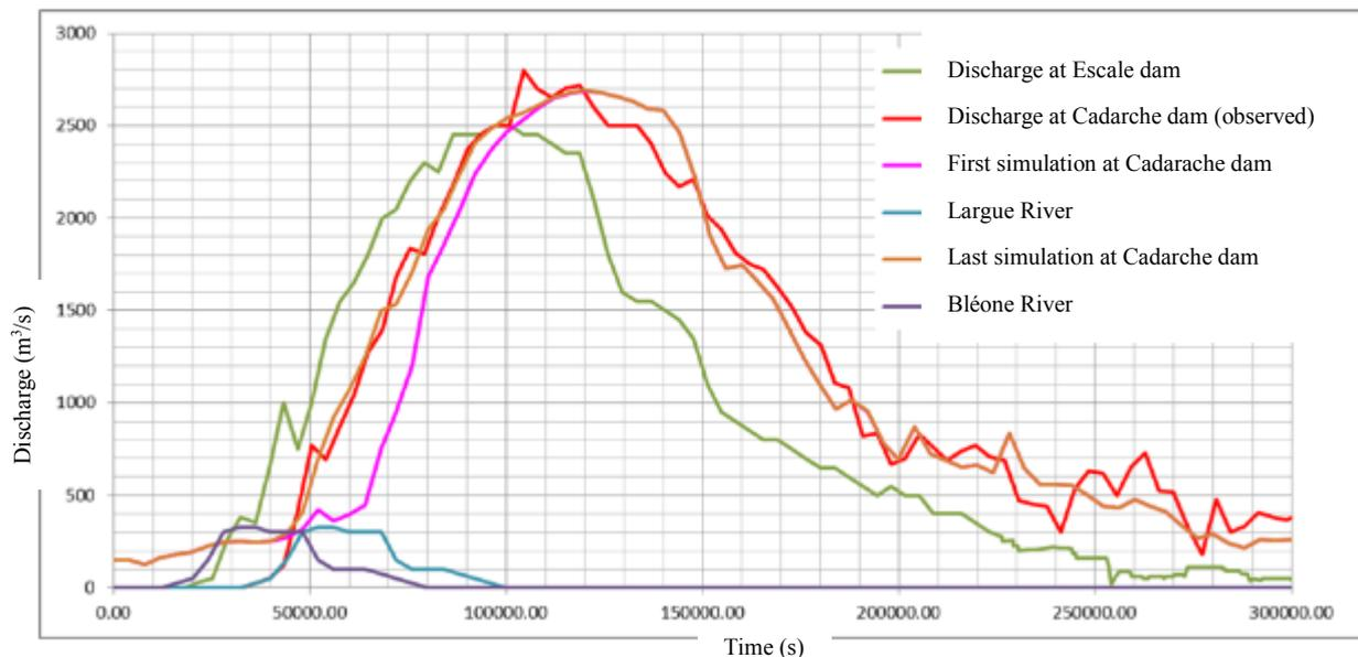
Figure 9. Model calibration of river section between Escale dam (green hydrograph) and Cadarache dam (red hydrograph) for historical flood of 1994 – Main tributaries: Largue and Bléone River
