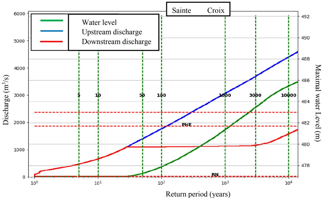
Figure 6. Water level (green), input discharge (blue) and output discharge (red) CDF for Sainte-Croix reservoir
