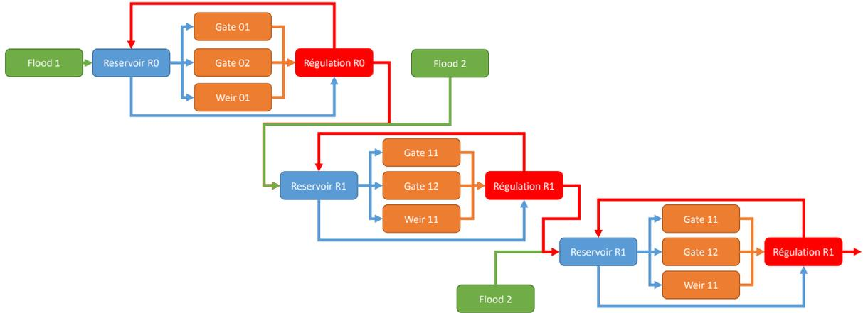
Figure 5. Melxor models of High Durance (up) and Verdon (down)
