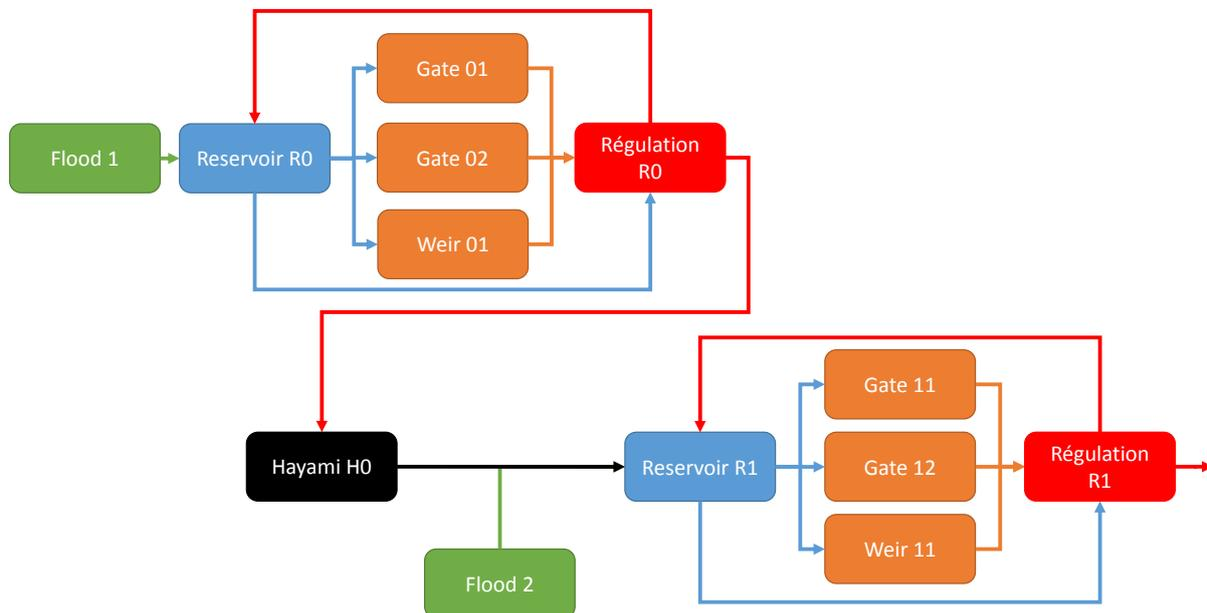
Figure 3. Example of Mel $\chi$ or model with two dams and Hayami propagation
